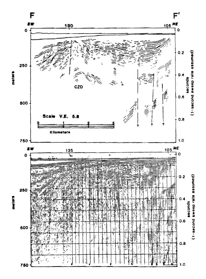
Figure 6.--Line drawing and seismic reflection profile of Woodward-Clyde Consultant's Line 816 showing CZD and deep faults nearshore. See Plates 1 and 2 for location.
