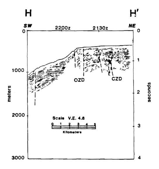
Figure 8.--Line drawing of USGS seismic reflection profile 33 (S2-78-SC) showing OZD and CZD. See Plates 1 and 2 for location.
