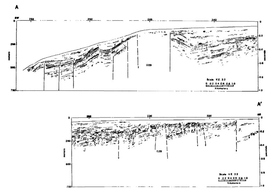
Figure 1.--Line drawing Marine Advisor's seismic reflection profile S-22 showing location of the OZD and CZD. See Plates 1 and 2 for location.
