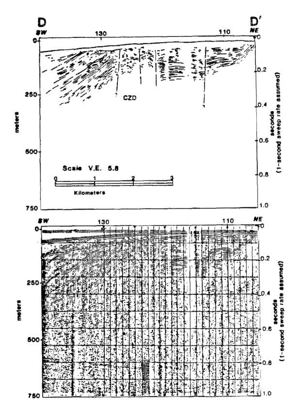
Figure 4.--Line drawing and seismic reflection profile of Woodward-Clyde Consultant's Line 822 showing CZD and inshore fault. See Plate 1 and 2 for location.
