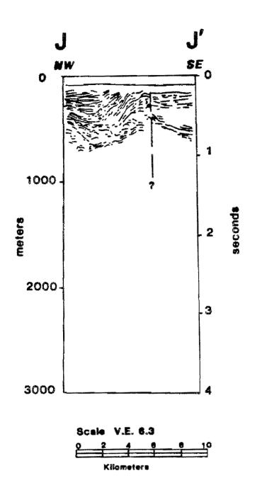
Figure 10.--Line drawing of USGS seismic reflection profile 57 (S2-79-SC) showing fault inshore of CZD. See Plates 1 and 2 for location.
