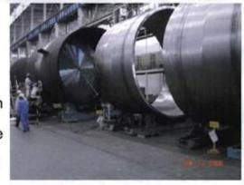
S/G 3A Lower and Middle Shell S/G 2A Balance Ring, Extension Ring, & Tubesheet
